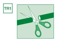
If necessary cut 9mm 3/8" pipe to a length suitable for your setup.
